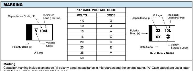
code for the voltage and EIA capacitance code.
